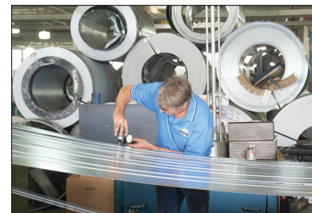
Quality control is a critical aspect of MTM’s operation. Above, a quality technician monitors the thickness of steel coil using a micrometer.
